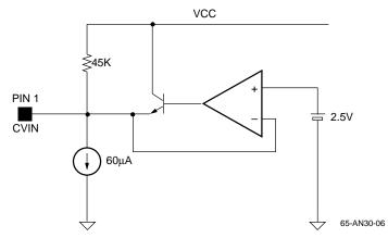
Figure 5. Input Structure for Sync Separator
