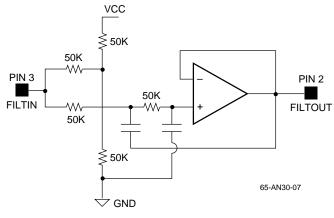
Figure 6. Input Filter Setup
