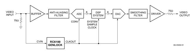
Figure 1. RC6100 Application in a Digital Video System
